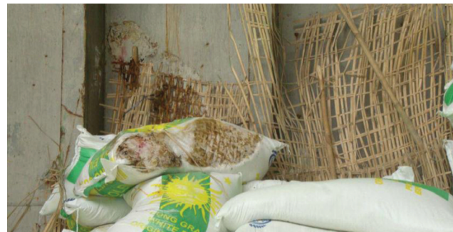
Bagged Rice Damaged as a result of Ship Sweat when in contact with Shell Plating in a Cargo Hold
