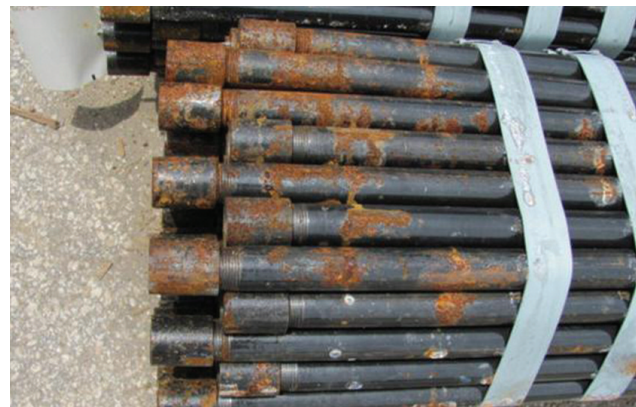
Steel Pipes Corroded as a result of Cargo Sweat
