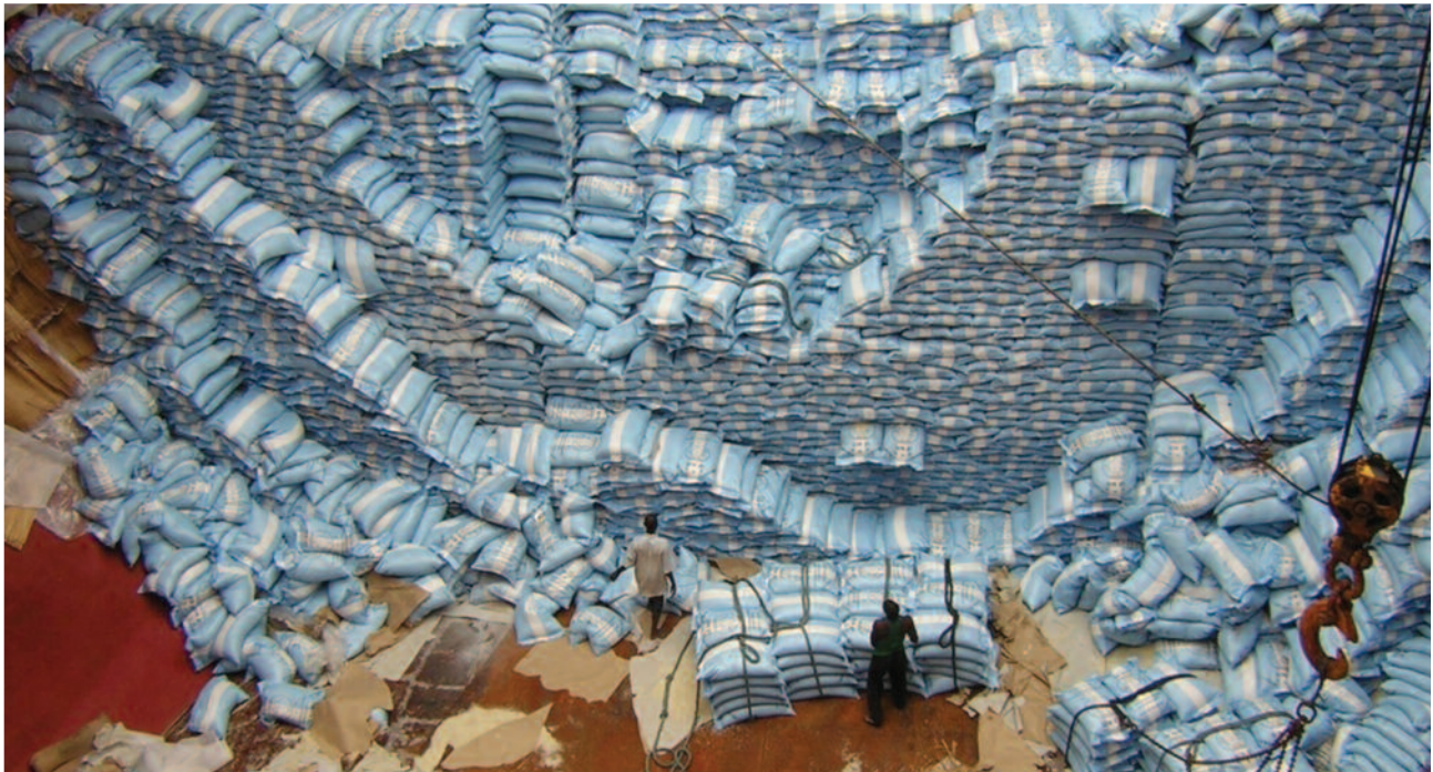
High unsupported cargo faces should be avoided due to the danger of collapse
