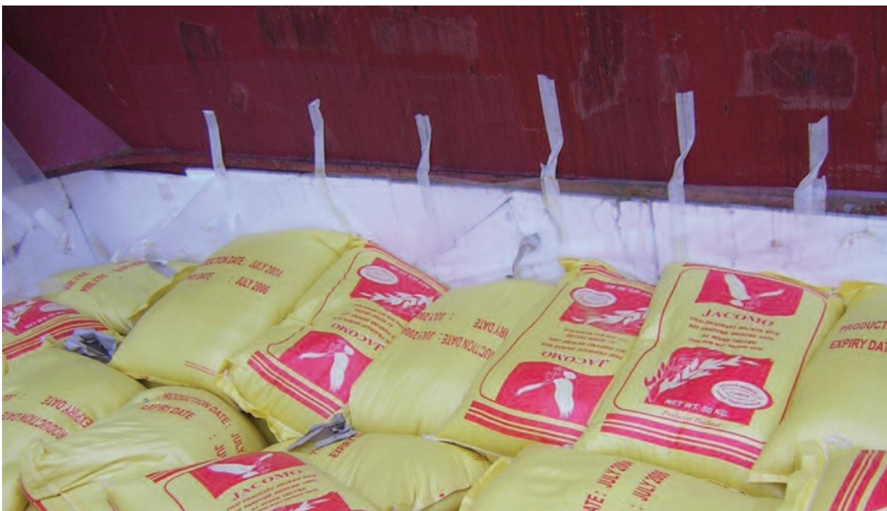
Styrofoam boards and plastic sheetting used in the Allied Maritime dunnaging arrangement
