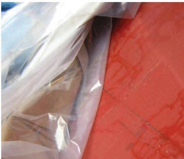
Moisture found behind plastic sheeting used in the Allied Maritime dunnaging arrangement
