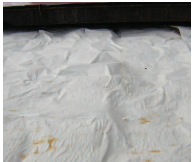
Kraft paper showing rust spots and signs of having been wetted and then dried
