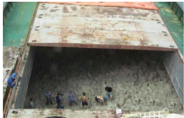
Bodily shift of cargo to starboard
