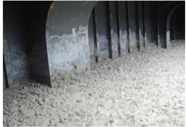
Cargo residues on steelwork inside hold indicating extent of cargo shift
