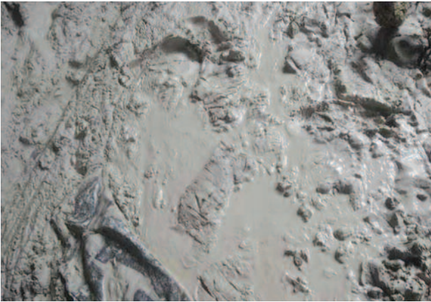
Appearance of the cargo surface after liquefaction
