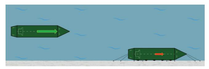
B. As the passing vessel starts to pass, the moored vessel will typically surge along the berth towards the passing vessel, sway away from the berth, and the end of the vessel furthest from the passing vessel will yaw towards the berth.
