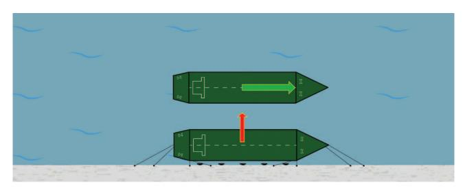
D. As the passing vessel starts to draw clear, the moored vessel will normally surge in the direction of travel of the passing vessel, will sway towards the berth and the end of the vessel closest to the passing vessel will yaw away from the berth.
