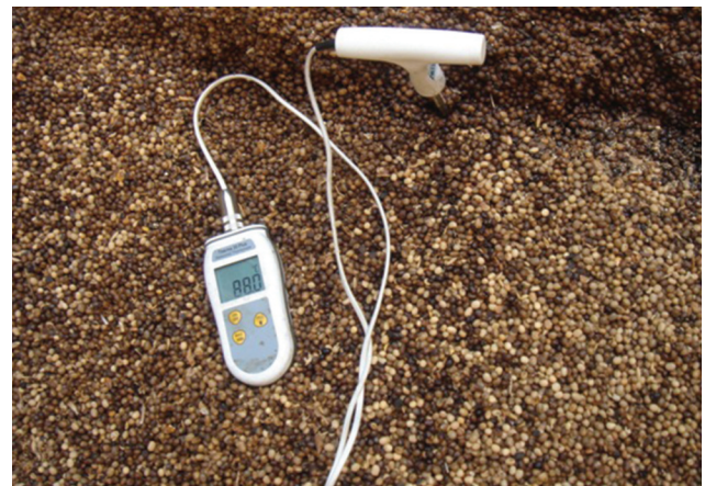
Self-heating of soya beans in contact with a heated fuel oil tank
