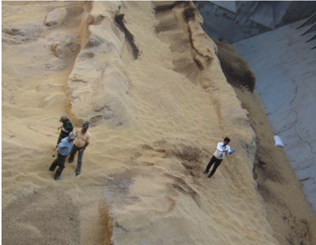
Clearly defined heat damage to soya beans in way of a centreline double bottom fuel oil tank
