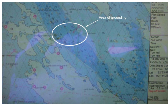
Chart view on 4,000 GT general cargo ship at a scale of 1:50,000; note the much greater detail in the area of the grounding. Photo: MAIB Report: Grounding of CFL Performer Haisborough Sand North Sea. © Crown Copyright
