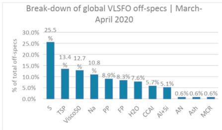
Of all the VLSFO's tested by VPS during March and April 2020, a global off-spec rate of 3.9% has been seen and does appear to be improving.
