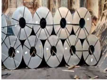
Lashing of coils
