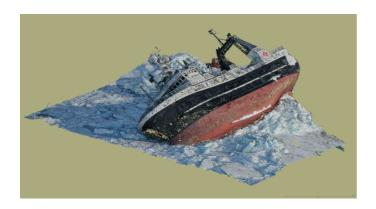
This is a 3D model of the grounded fishing vessel 'Northguider' created using photogrammetry from a drone
