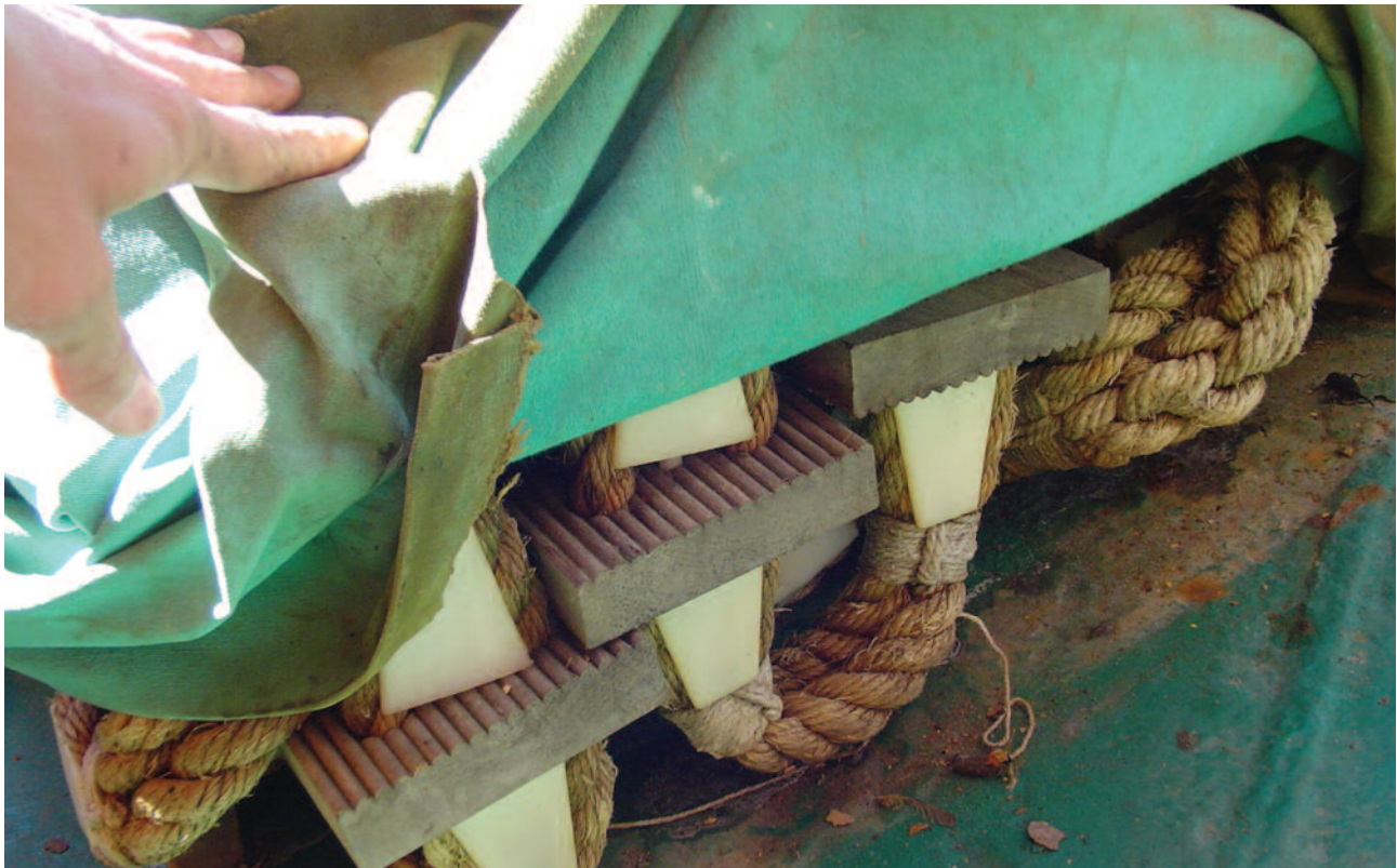
An embarkation ladder resting on deck exposed to attack by water and cleaning chemicals
