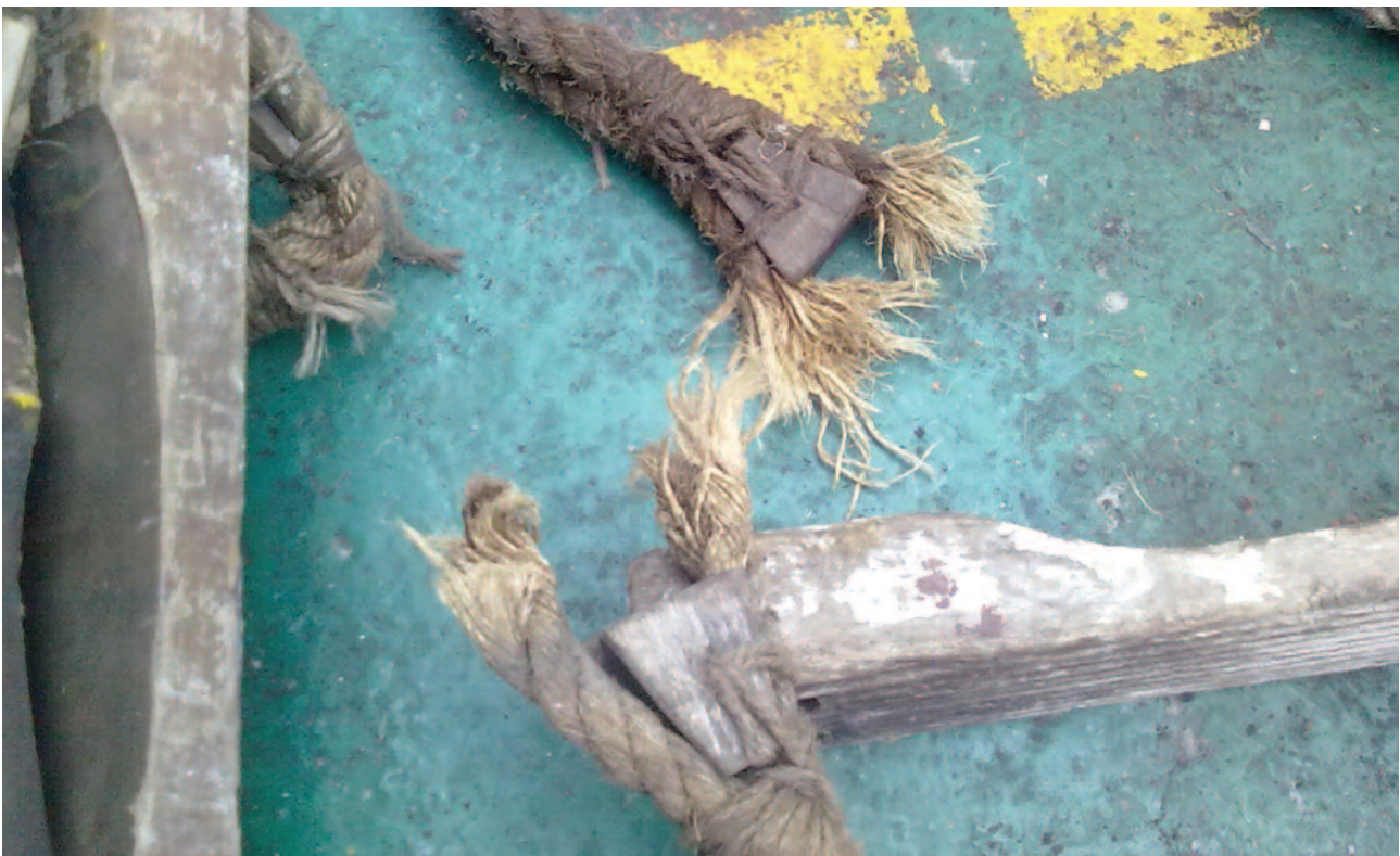
A pilot ladder side rope which failed as a pilot climbed the ladder
