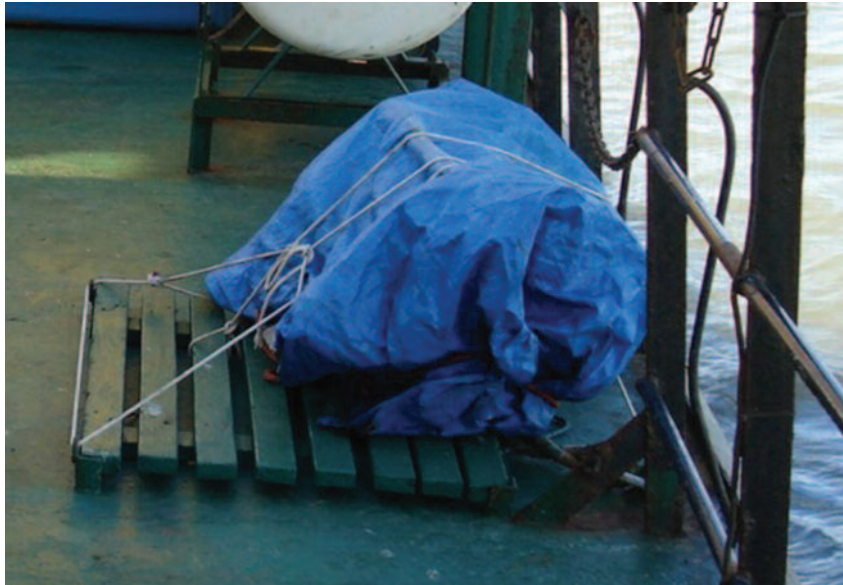
An embarkation ladder stowed clear of the deck and suitably covered
