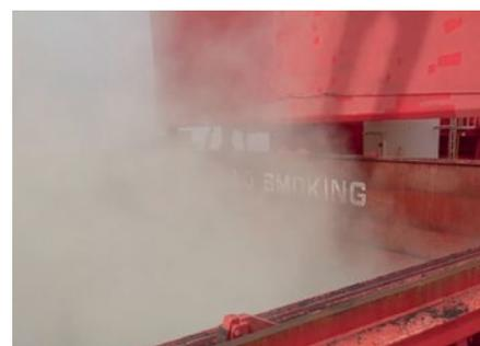
**Coal self-heating in the cargo hold despite being cooled below 55°C on the barge prior to loading.**
