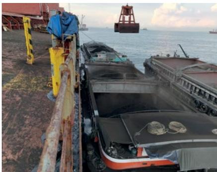
In most cases, coal loaded in Kalimantan is from barges and the Club has noticed a growing trend of increased pressure from shippers to load cargo from barges where temperatures in excess of 55°C have been recorded.
