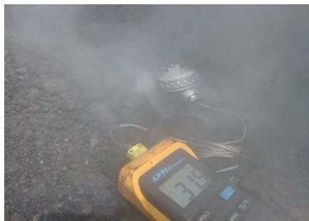
**Coal on a barge measured to be below 55°C but clearly self-heating as evidenced by the smoke/steam.**
