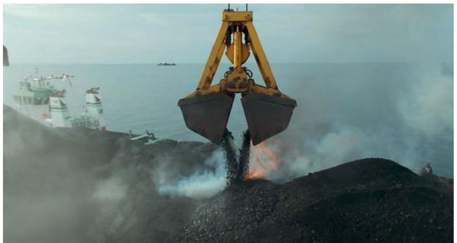
Turning hot coal over on a barge to try and cool it.
