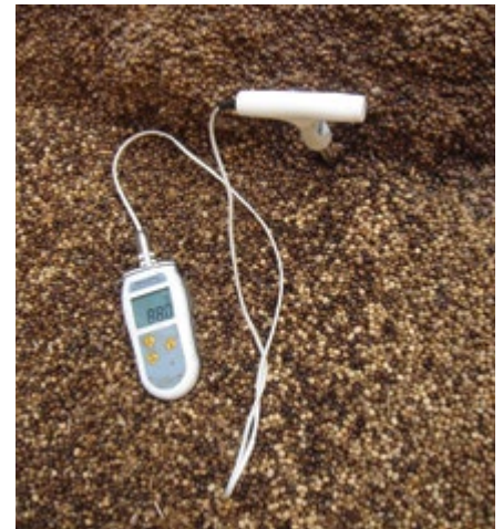
Self-heating of soya beans in contact with a heated fuel oil tank
