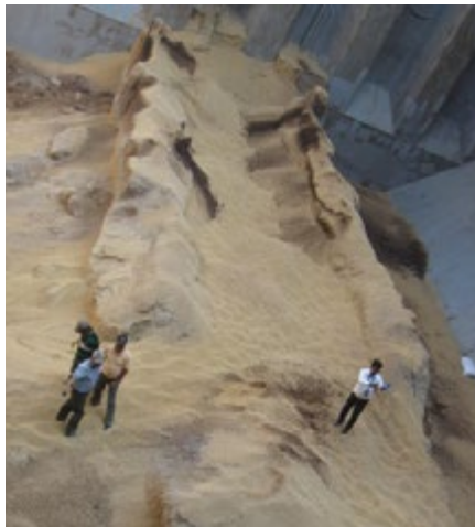
Clearly defined heat damage to soya beans in way of a centreline double bottom fuel oil tank
