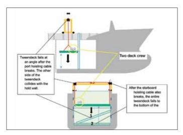
The port hoisting cable broke and the port side of the tweendeck fell to the bottom of the hold, damaging the starboard side of the hold wall and sending the two crew tumbling to one side. The starboard hoisting cable then also broke, and the entire tweendeck fell to the bottom of the hold.
