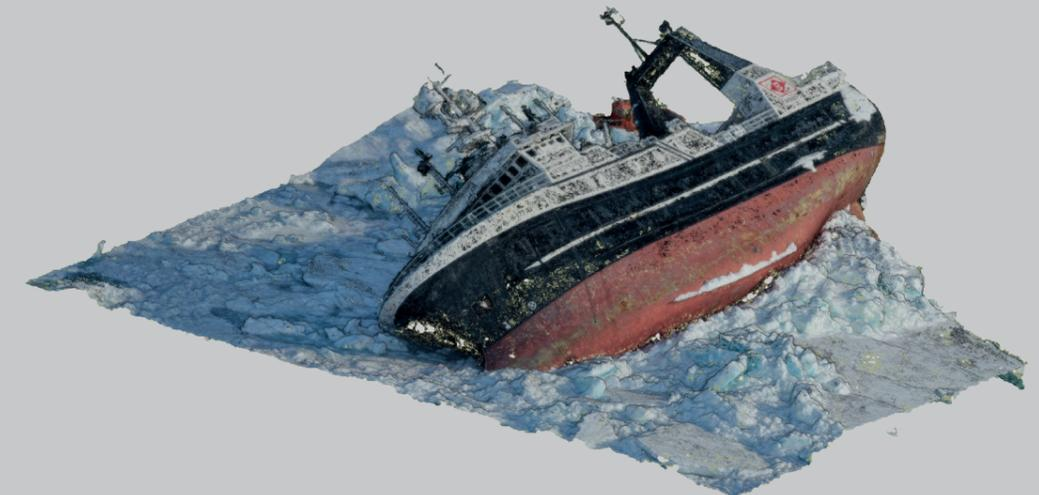
This is 3D model of the grounded fishing vessel 'Northguider' created using photogrammetry from a drone
