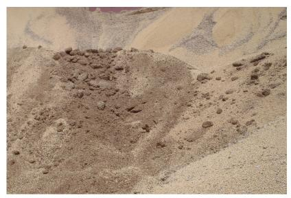
Caking due to cargo being next to a heated double bottom fuel oil tank
