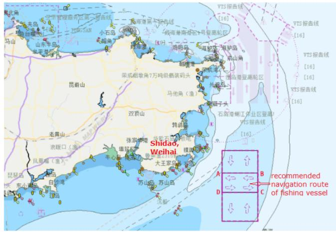
This recommended route spans 11 nautical miles from east to west and 6 nautical miles from north to south. It is intended to guide fishing vessels through the densely navigated area in southeast of Shidao in an orderly manner, thereby regulating the navigation order of this area and preventing potential collisions between commercial and fishing vessels.
