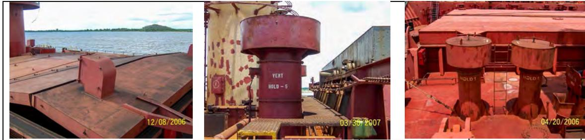
*Figure 16: Photo collage of typical ventilators on hatch covers*
