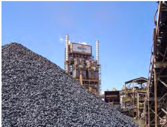
Figure 7: Open stockyard storage of HBI
