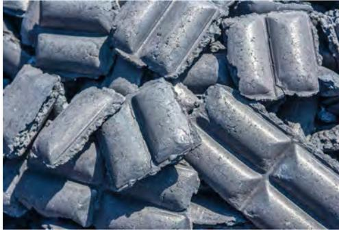
*Figure 1: Hot Briquetted Iron
