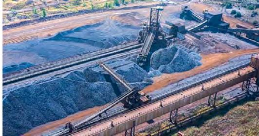
Figure 4: Travelling conveyor-stacker and bucket wheel reclaimer at HBI Plant yard
