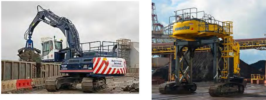
*Figure 6: Railcar loaders having "soft-loading" capability (to minimise drop height)
