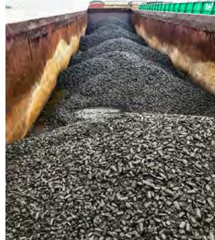
Figure 22: Correct loading of HBI to barges
