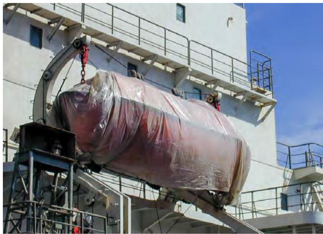
Figure 21: Protecting vessel equipment from HBI dust
