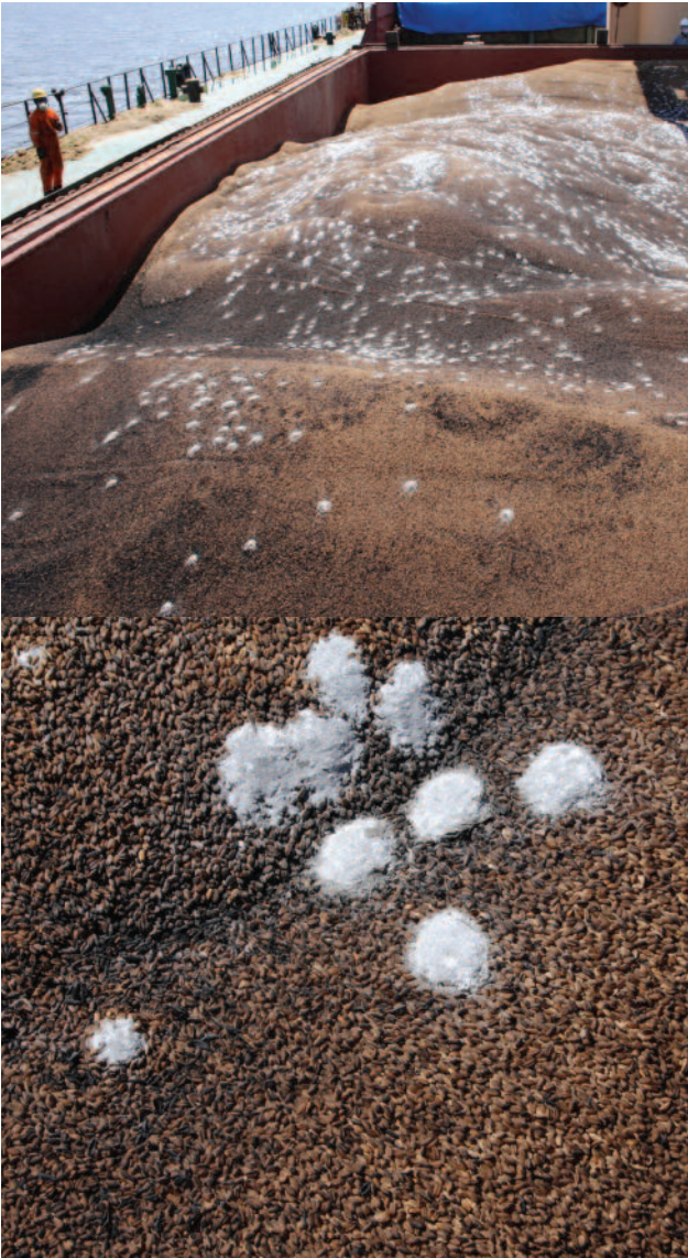
Heat damaged cargo with remaining tablet/pellet residues
