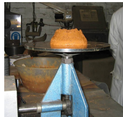
Flow table test of nickel ore (Photo: Brookes Bell)
