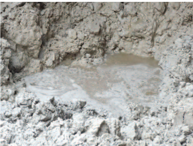
Condition of the flourspar after liquefaction
