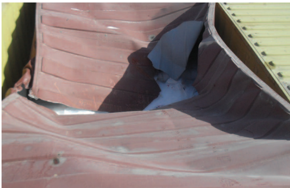
Hoist wire failure caused a crane block to fall on to this loaded container, causing considerable damage
