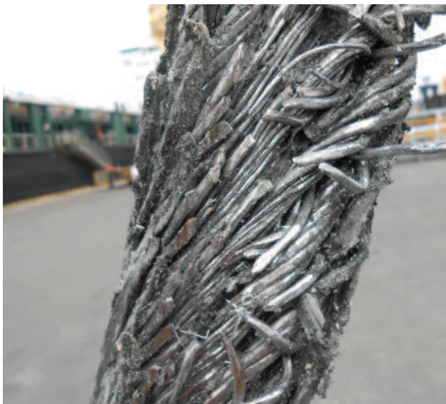
Heavily damaged hoist wire
