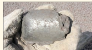
◀ Figure 1: DRI (A), Briquettes, hot moulded (also referred to as iron ore briquettes, briquetted iron ore)
