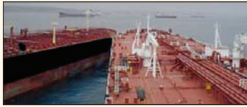
▲ Contact occurred when mother vessel (black hull) yawed to starboard during approach
