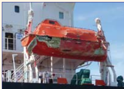
◀ Lifeboat damaged by manoeuvring tanker's anchor
