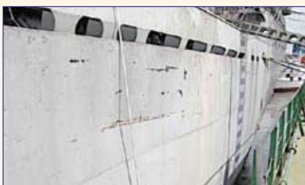
◀ Cement vessel's side shell dented and scratched
