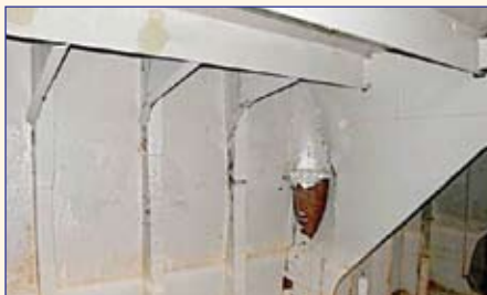
◀ Cement vessel's side shell dented and scratched
