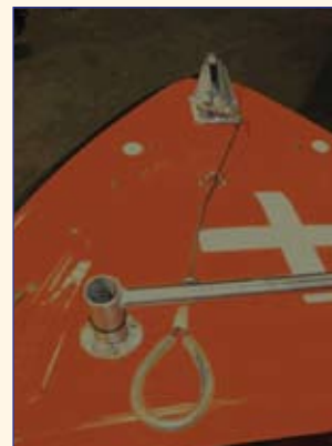
▲ Original design showing painter release lanyard situated under the forward grab rail
