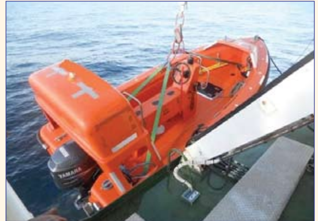
▲ Rescue boat prior to launching showing forward painter secured
