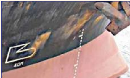
▶ Cement vessel's side shell holed and internals damaged by bulk carrier's anchor
