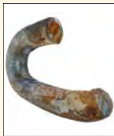
▲ Broken link of chain later recovered from deck
