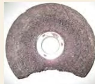
View of broken rotary cutting disk – the missing segment which was flung at high speed could easily have caused very severe injury to the crewman or other personnel in the vicinity
