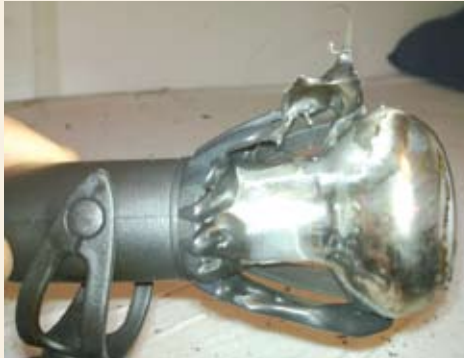
The detached clamp-on spotlight with partly melted shield and exposed bulb
