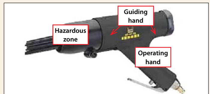
Typical compressed air-operated needle hammer gun with pistol grip showing safe and hazardous hand grip areas
