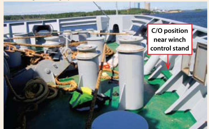
C/O was standing in snap back zone when rope parted
