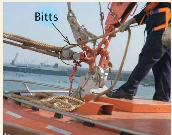
the coach roof and secured to bitts welded to the bowsing tackle blocks fitted to the lifeboat lifting plates.
