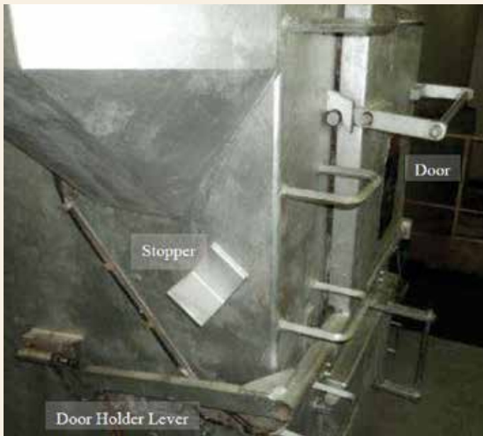
Incinerator with door closed
