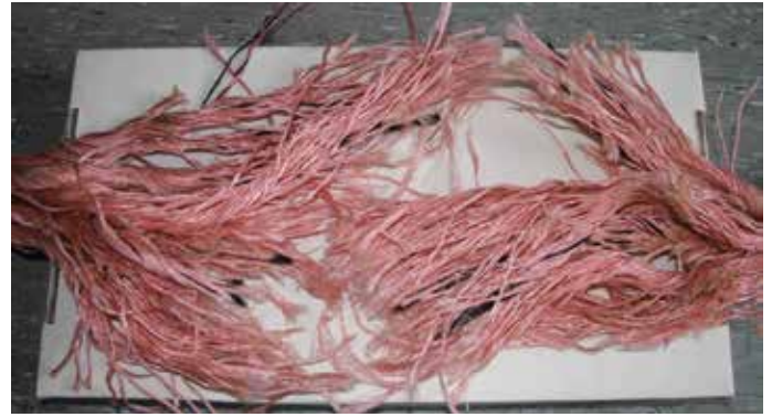
Failed stretcher, subsequently found to be undocumented and of unknown manufacture or SWL
