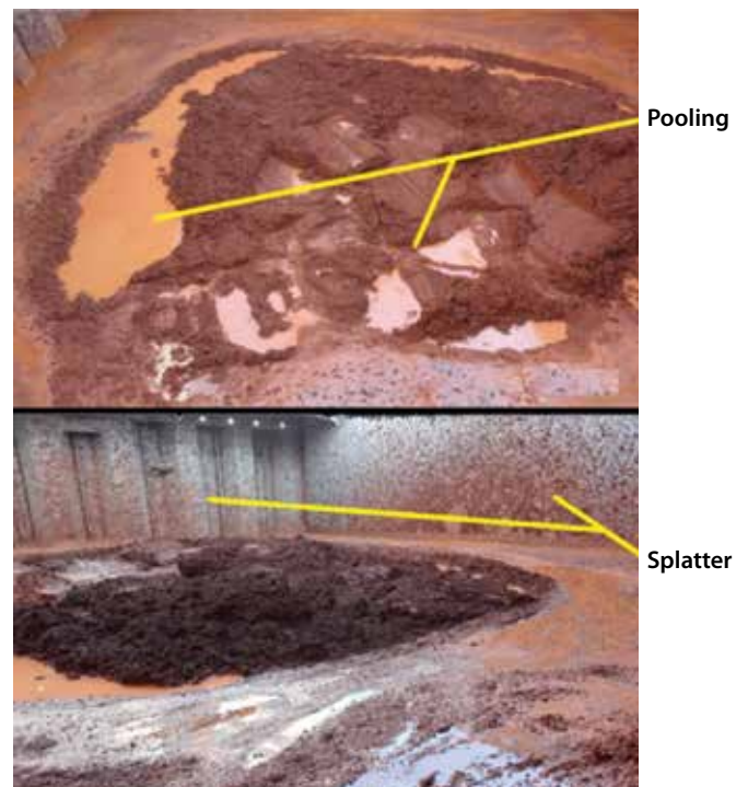
View of bauxite cargo loaded on another vessel at the same port at about the same period as the casualty vessel
