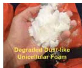
Degraded Dust-like Unicellular Foam
