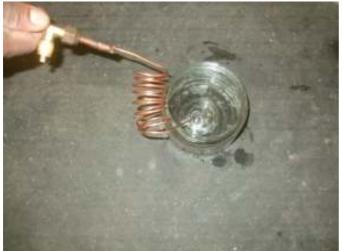
To minimise the risks associated with flammable gases and to comply with F-gas regulations, use a set of service gauges and a capillary as shown.
