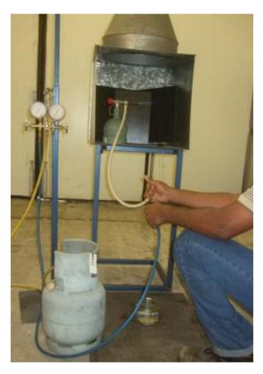
To minimise the risks associated with the product of degradation fumes, fabricate a fume cupboard using an enclosure and extractor fan.
