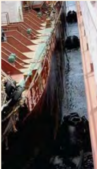
Large bunker vessel on left rigged with three undersized fenders
