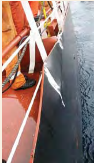
View of contact damage near the tanker's stern
