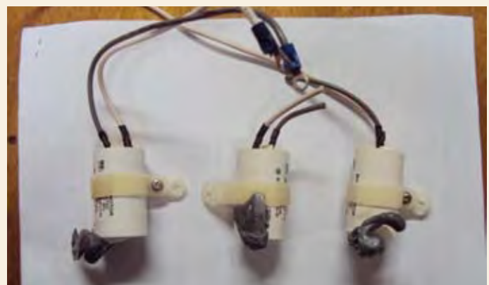
Other capacitors that have overheated with expelled electrolyte
