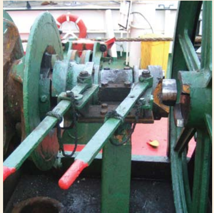
Broken dog clutch and bent shaft on port windlass
