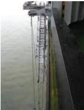
The damaged telescopic accommodation ladder from which a seaman fell to his death when the hoist winch failed (Courtesy MAIB)
