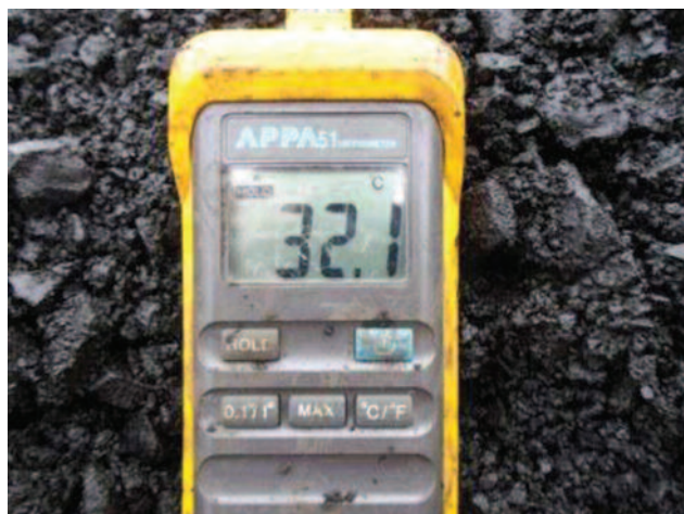
Coal temperature monitoring by temperature probe
