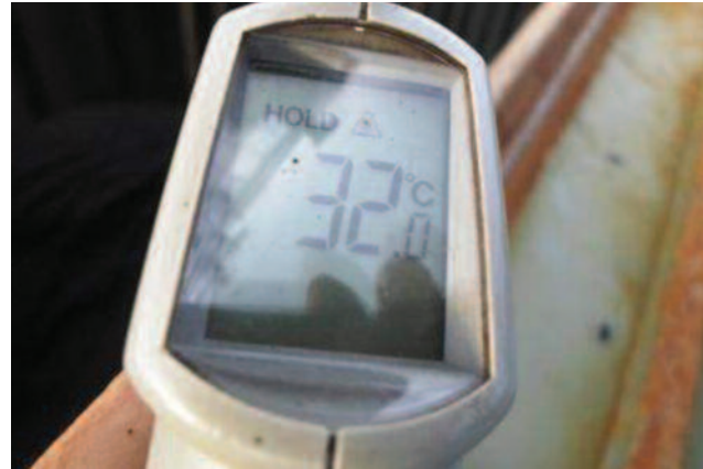
Coal temperature monitoring by infrared thermometer
