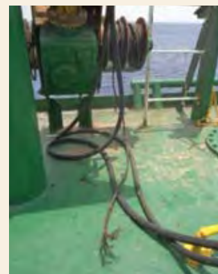
View showing parted fall wire and gangway winch with multiple drums
