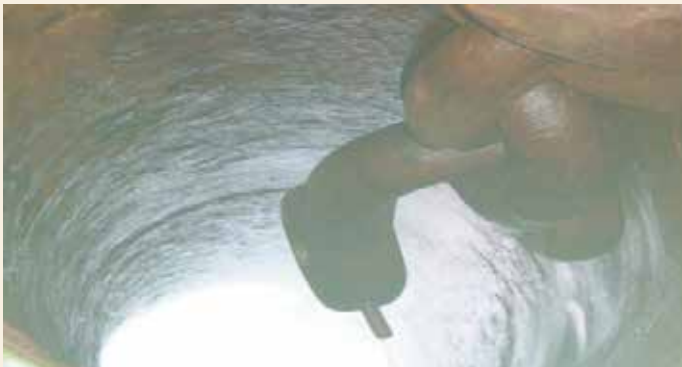
Missing starboard anchor
