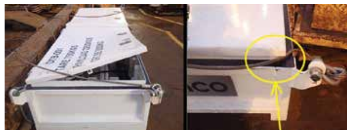
Lifting bridle snagging the lid
